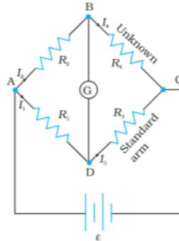
Meter bridge works on the principle of a balanced wheatstone bridge.
